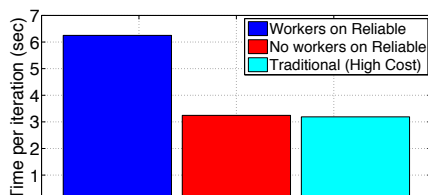
Figure 13: AgileML stage 3 (red) with 1 reliable and 63 transient compared to stage 2 (same ratio; blue) and traditional.
